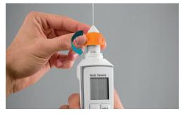
a. To change the probe, twist the orange probe base counter clockwise until the attached probe releases.
